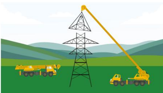
Stage 3: Building pylons
