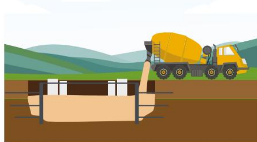
Stage 2: Pylon foundations
